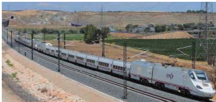
RENFE Serie 730 trains Electric AC DC – Diesel Double gauge 1668-1435 mm
